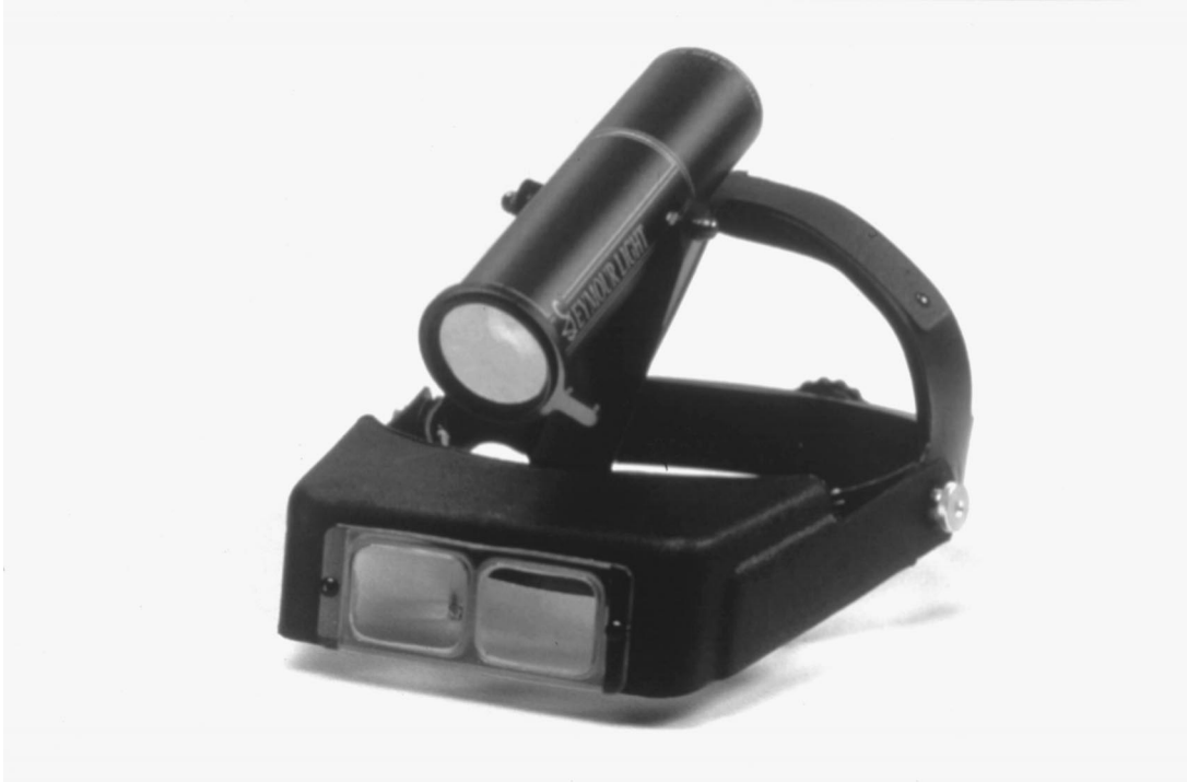
Figure 5. A magnified polarizing headlight is used to more clearly contrast the individual vessels.
